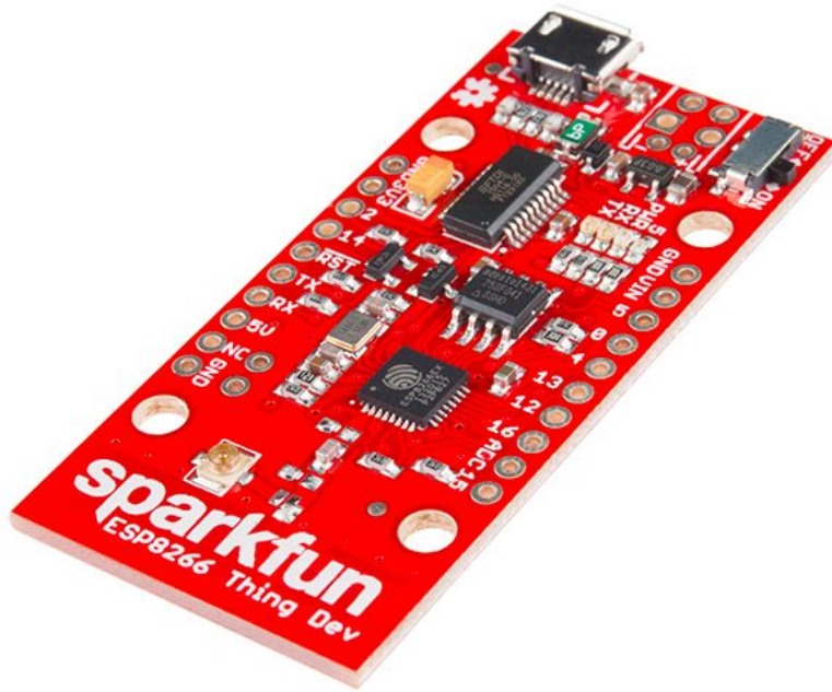
Figure 1. Sparkfun ESP8266 Thing Dev
